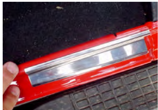
Passenger side rear 4door version. Note how it is poisoned and also the taper of the guard Wide side to the front, small side to the rear.
