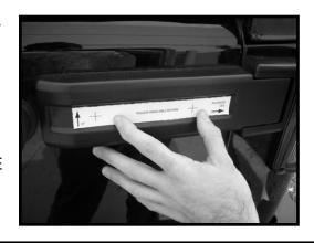
2. Install lower mounting plate by first removing the (2) lower tailgate hinge bolts. If installing on a vehicle with a RR tire carrier, use (2) M8 bolts with (2) 25mm spacers to secure the lower mounting plate to the tailgate as shown. (3) flat washers should be used for each bolt. Place (1) under the bolt head and (1) on either side of the spacer.
