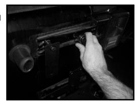
If no RR tire carrier is present, rotate the bracket installed in step 2 into its vertical position and the upper mounting plate into its horizontal position. Line up the holes in the plate and the bracket with the upper right tailgate hinge hole. Tighten the bracket into place using the remaining M8 hardware as shown. Also, fully tighten the bottom right tailgate hinge bolt.
