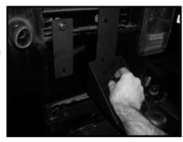
If installing Off Road Mounting Bracket without a RR tire carrier, install the final M10 bolts into the bottom holes in the mounting bracket as shown. Go back and make sure all bolts are tightened before inserting your Off Road Jack.
