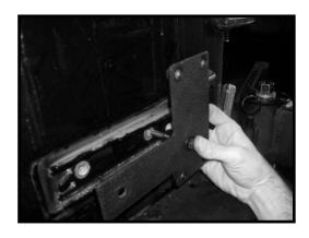
If installing on a vehicle without a RR tire carrier, the mounting bracket should be installed with the lower mounting plate in this step. Line up the bottom M8 hole with the bottom right tailgate hinge bolt hole and insert M8 hardware as shown. Do not fully tighten the bolt securing the mounting bracket. The mounting bracket will have to be rotated to gain access to the upper right tailgate hinge bolt in the next step.
